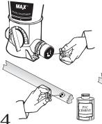
Following PVC cement directions brush PVC cement on to ends of pipe and the inside of bushings.
