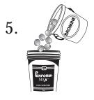
Fill unit to top with chemical. DO NOT MIX BROMINE AND CHLORINE. Do not put small particles in feeder. Always wear protection for eyes, skin and clothing. Avoid sparks, open flame or smoking when handling chemicals.
