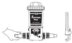
2. Screw adapters into each end of Perform-Max. Tighten turning
