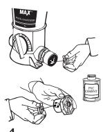
Following PVC cement directions, brush PVC cement on reducer bushings and inside of male adapters.
