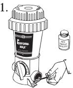
Following pipe thread sealant directions, brush sealant onto Perform-Max threads in both ports.
