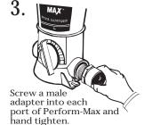
Completely tighten turning 1 to 2 revolutions with a wrench. DO NOT OVERTIGHTEN.
